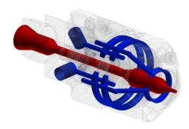
The pneumatically controlled nozzle type NE has a needle shut-off mechanism which stops the melt stream directly at the mold interface. Rubber, liquid silicone rubber and other elastomers can be processed without fear of premature vulcanization due to the nozzle's integrated cooling system, which uniquely regulates temperature through the entire nozzle. The nozzle can also be fitted with an interchangeable diving tip for cold channel applications.
